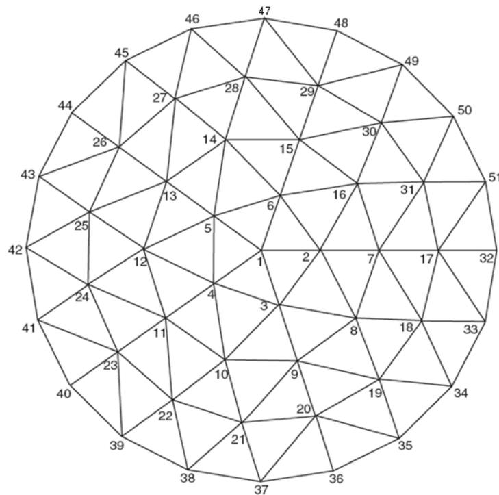
Figure 3. Plan view of a geodesic dome.
