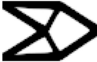
Figure 6. Optimum layout by SIMP and FEM [33]
