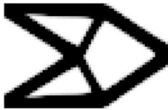
Figure 6. Optimum layout by SIMP and FEM [33]
