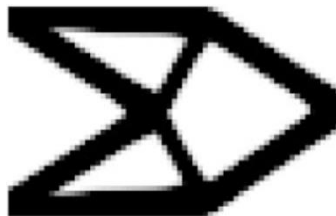
Figure 5. Optimum layout by SIMP and FEM [3,27]
