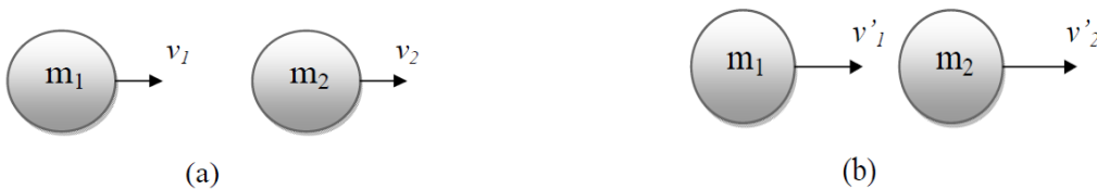
Figure 2. The collision between two bodies; (a) Before the collision. (b) After the collision
