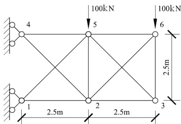
Figure. 4 The 10-bar plane truss structure
