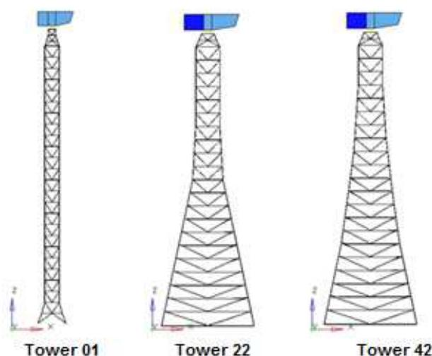
Figure 3. Advancement project freestanding lattice tower wind
