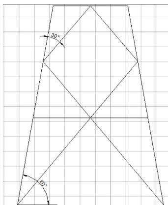
Figure 17. Angle position of the optimum lattice tower
