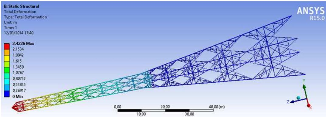
Figure 15. Total deflection due to loads in ANSYS®
