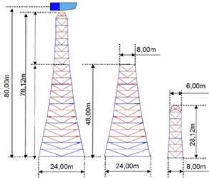
Figure 2. Representation of the lattice wind tower
