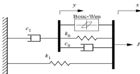
Figure 1. Simple mechanical model of the MR damper
