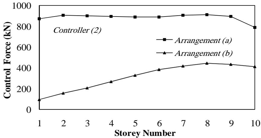
Figure 12. The maximum control force when using Controller (2)
