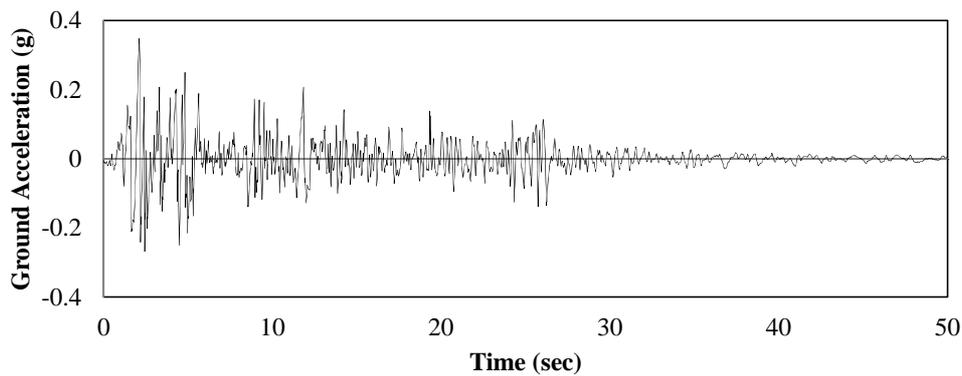
Figure 4. Ground acceleration of the 1940 El-Centro earthquake
