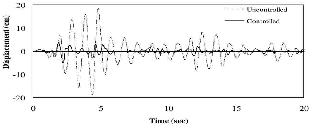
Figure 10. Time history of the 10<sup>th</sup> floor displacement
