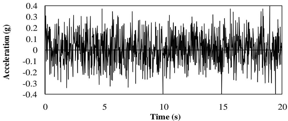
Figure 13. Ground acceleration of the White noise excitation
