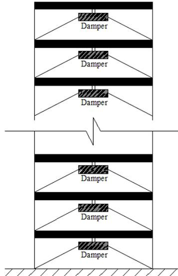
Figure 3. 10-storey shear frame equipped with 10 MR dampers
