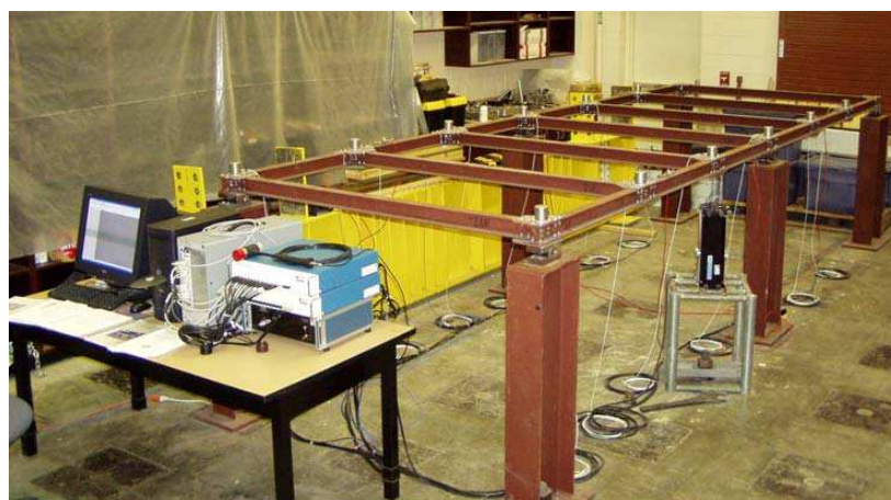
Figure 8. Steel bridge benchmark [28]
