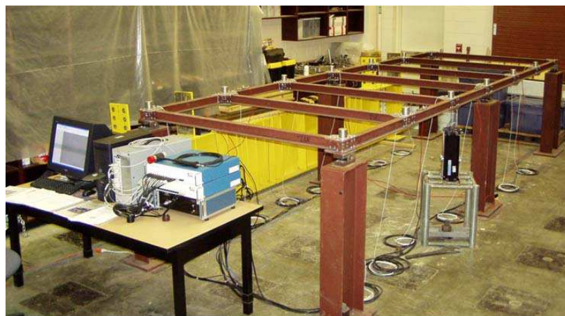
Figure 8. Steel bridge benchmark [28]
