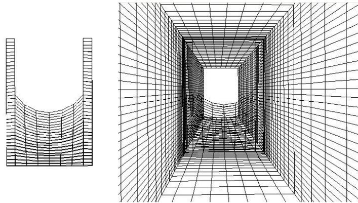
Figure 2. weir model and meshes in gambit software (b= 20 cm)
