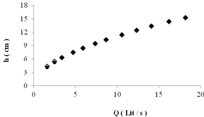
Figure 6. Ratio of flow rate variations - water head for contracted compound arched rectangular sharp crested weir  $b=20$  (cm),  $h_0=7.5$  (cm)
