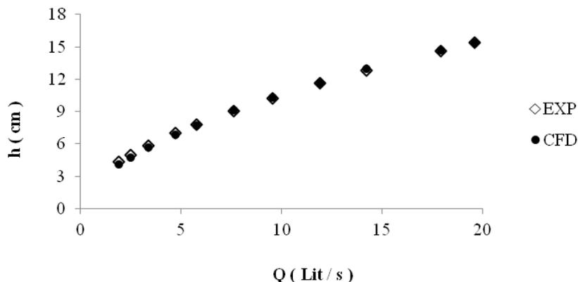
Figure 7. Ratio of flow rate variations - water head for contracted compound arched rectangular sharp crested weir  $b=20$  (cm),  $h_0=5$  (cm)
