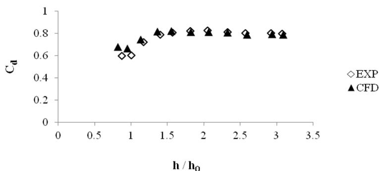
Figure 10.  $C_d$  changes in contracted compound arched rectangular sharp crested weir  $b=20$ (cm),  $h_0=5$  (cm)
