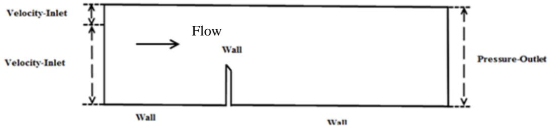
Figure 4. Boundary conditions imposed on the model
