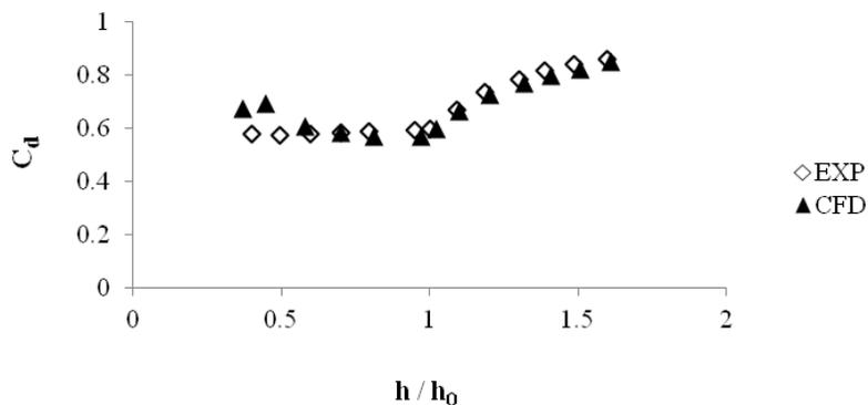
Figure 8.  $C_d$  changes in contracted compound arched rectangular sharp crested weir  $b=20$  (cm),  $h_0=10$  (cm)
