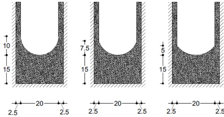
Figure 1. Sections of arched rectangular sharp crested weirs ( $b = 20$  cm)
