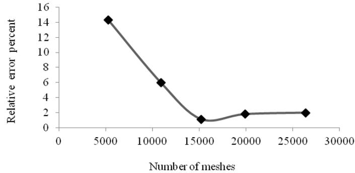
Figure 3. Relative error ratio of water depth in upstream of the weir crest for different amounts of meshes
