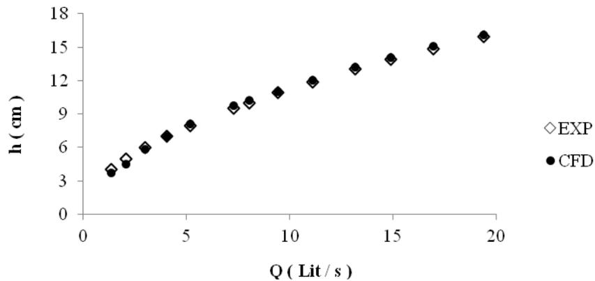
Figure 5. Ratio of flow rate variations - water head for contracted compound arched rectangular sharp crested weir  $b=20$  (cm),  $h_0=10$  (cm)
