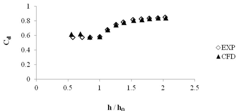
Figure 9.  $C_d$  changes in contracted compound arched rectangular sharp crested weir  $b=20$  (cm),  $h_0=7.5$  (cm)
