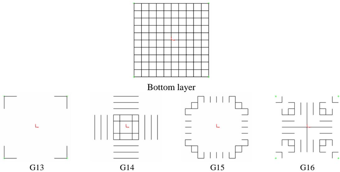
Figure 7. Member grouping details of the bottom layer for the 968-bar double layer grid
