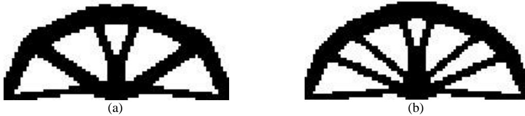
Figure 15. The comparison of the final optimal topology based on (a) FEM and (b) IGA
