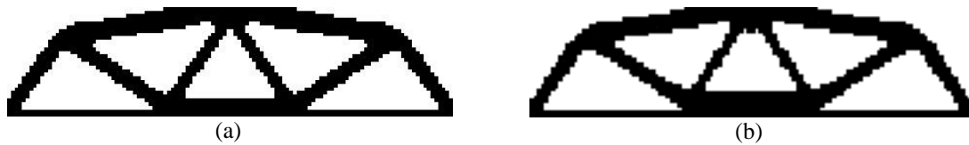
Figure 9. The comparison of the final optimal topology based on (a) FEM and (b) IGA
