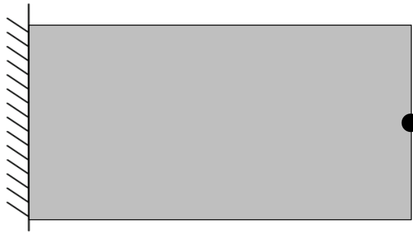
Figure 4. A rectangle cantilever beam
