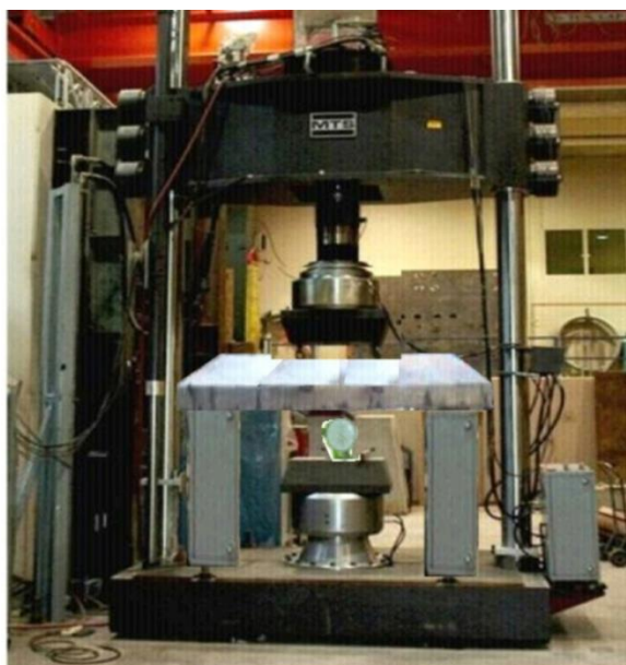
Figure 2. Experimental setups for Load-Deflection test on 700x600mm slab
