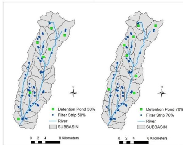
Figure 5. BMPs distribution for 50% and 70% reduction cases
