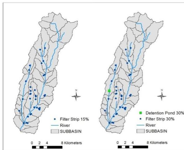
Figure 3. BMPs distribution for 15% and 30% reduction cases
