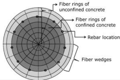
(c) Fiber sections used at hinge locations
