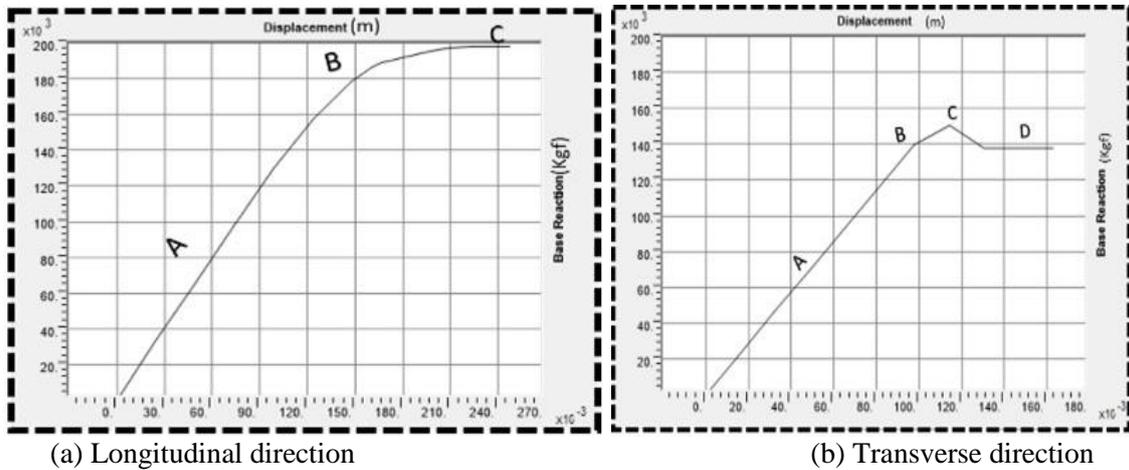
Figure 8. Pushover curve for optimum quasi-isolated bridge
