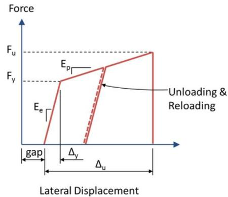
Figure 5. Force-Displacement model for retainers
