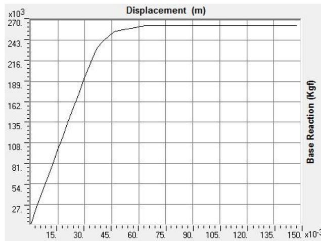
Figure 9. Transverse pushover curve for optimum conventional bridge
