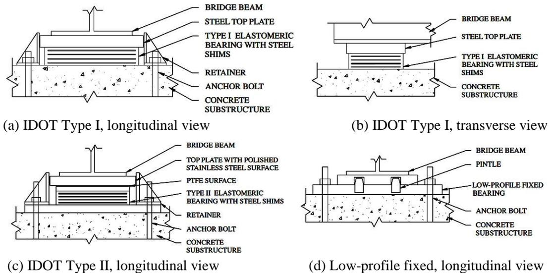
Figure 1. Bridge bearing types under consideration [29]
