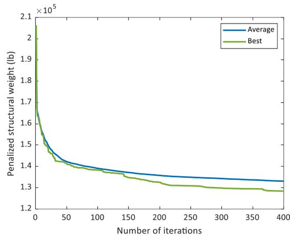
Figure 6. Convergence curves of the ACSS corresponding to the best result and the average of results obtained from 20 runs for the planar ten-story frame
