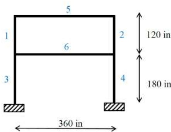
Figure 1. Geometry and member numbering of the planar two-story frame
