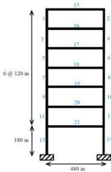
Figure 3. Geometry and member numbering of the planar seven-story frame
