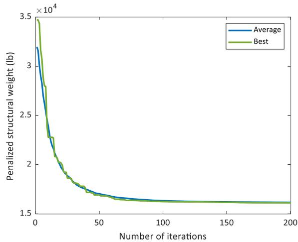
Figure 4. Convergence curves of the ACSS corresponding to the best result and the average of results obtained from 20 runs for the planar seven-story frame
