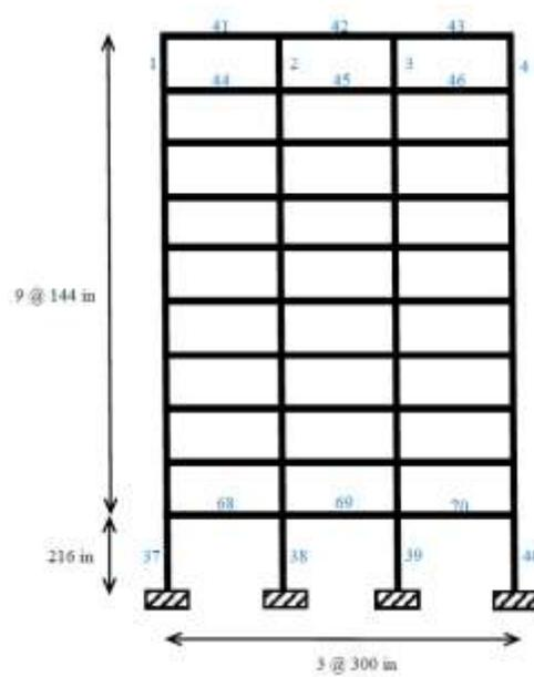
Figure 5. Geometry and member numbering of the planar ten-story frame
