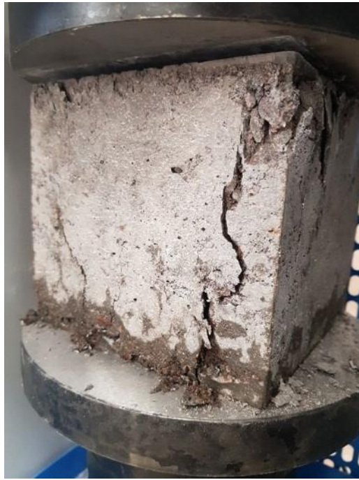
Figure 3. Failure of a concrete specimen
