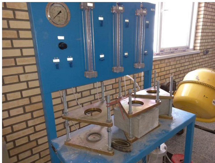
Figure 17 An image of the permeability test apparatus
