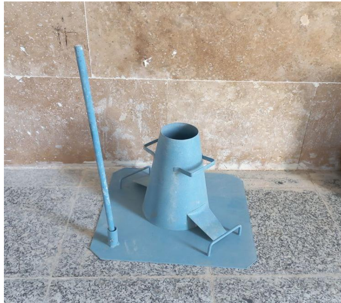
Figure 10. Slump test cone
