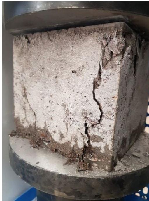
Figure 3. Failure of a concrete specimen
